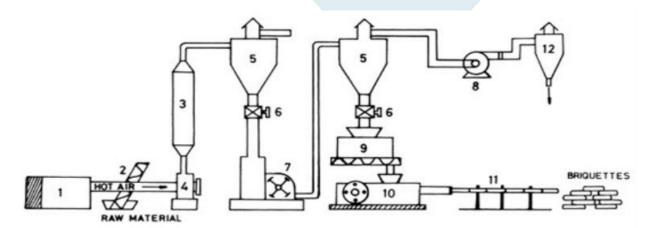
1-furnace/hot air generator 5-cyclo 2-inclined screw feeder 6-air lo
