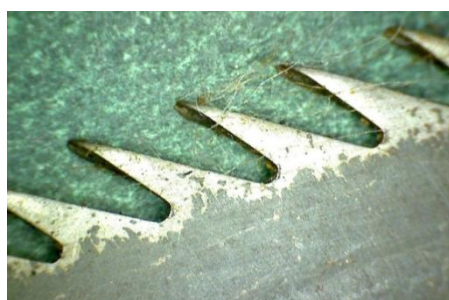
Rice. 2. Gripping ability of saw blade teeth: untreated (a) and treated with an abrasive flow (b)
