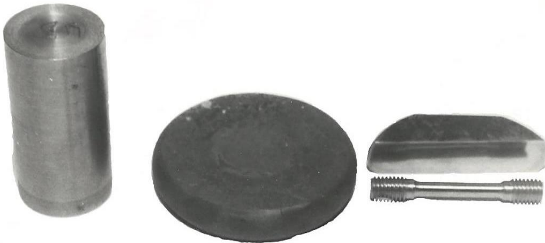
Figure 2.3. Samples for upsetting, used for tensile mechanical testing and microstructural investigations.
