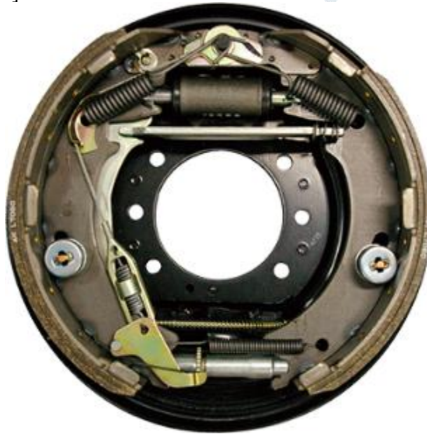
Figure 6. Duo-servo type drum brake
