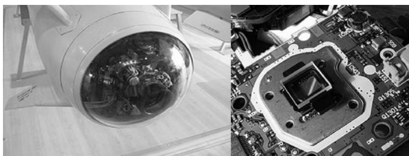
Fig. 1. The Kh-59 "Ovod" missile's television seeker and matrix photodetector
