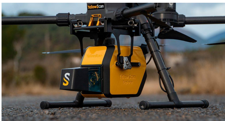
Figure 3. Drone with LiDAR Sensor
