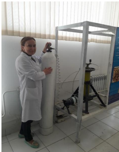
Fig. 5. Laboratory equipment for studying the process of extracting ingredients from plant material using CO 2 .
