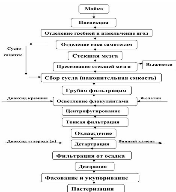
Figure 1 - Flow chart of grape juice production
