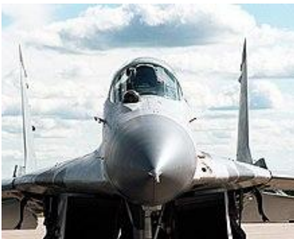
Pic.7 MiG-29 nose showing radome and S-31E2 KOLSIRST
