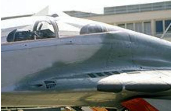
Pic.8 MiG-29UB on display, showing gunport
